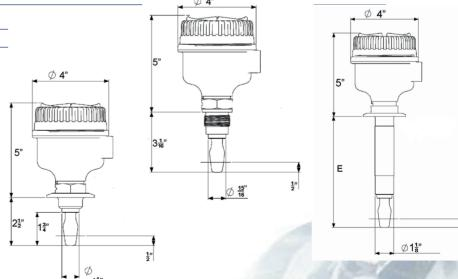
Options: Hand polished wetside to a finish better than 0.8µm meets the principle design criteria of 3A and EHEDG
