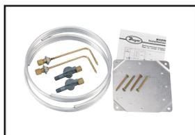
Air Filter accessories furnished are mounting panel with necessary screws, two static pressure tips with integral compression fittings, two five foot lengths of 1/4” aluminum tubing and the two molded plastic vent valve with compression fittings.
