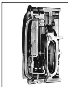
Cutaway view of the Magnehelic® gage showing the actuating diaphragm, the leaf spring with magnet, the helix which turns the indicating pointer in response to the position of the magnet without mechanical linkages.
