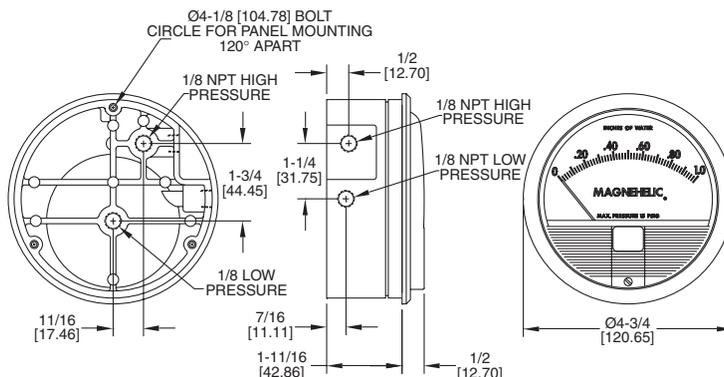
The Magnehelic® gage consists of two pressure-tight compartments separated by a molded flexible diaphragm.
