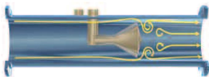
*The V-Cone's contour-shaped cone directs the flow without impacting it against an abrupt surface and minimizes headloss. As a result, the beta edge of the cone is not subject to wear by dirty fluids. Because it remains unchanged, V-Cones rarely, if ever, require recalibration.*
