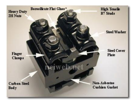
After the gage is placed in service and becomes thoroughly heated, expansion of metal parts causes bolting pressure to ease somewhat. Close water gage valves and go over nuts and tighten them to correct torque value. For cleaning and/or replacing the flat glasses and mica protectors, remove gage from gage valves and follow this procedure:
